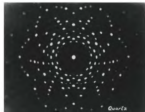
(b) Laue diffraction pattern for a thin section of quartz crystal
